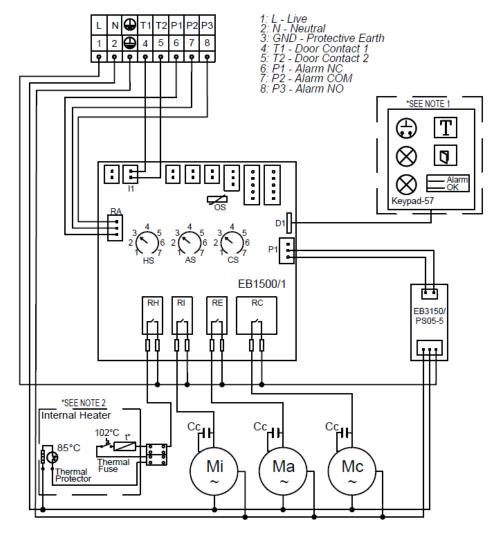
Part List: Mc: Compressor Ma: Ambient Fan Mi: Internal fan Ci: Internal Blower Capacitor Ca: Ambient Blower Capacitor Cc: Compressor Capacitor
